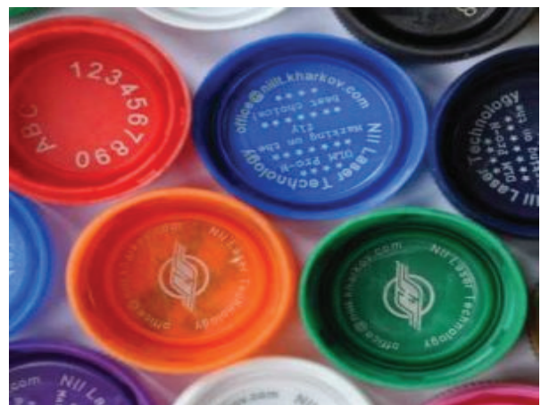
Laser coding provides a simple way to print onto a screw cap.
